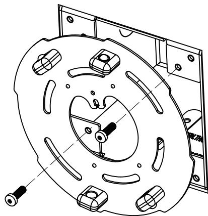
1. To secure installation bracket of fixture to square housing with screws.
