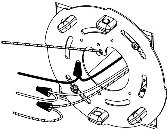
3. Make the wire connections. The green(ground wire) of housing to green of fixture, Female connection of housing to male connection of fixture.
