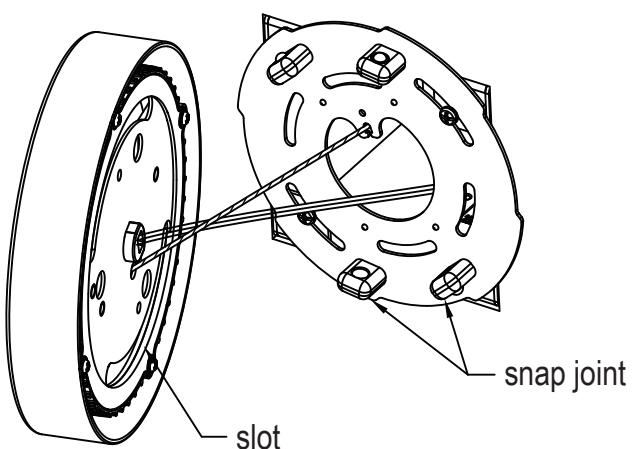
4. Push and feed all wires up into Junction Box as you raise the fixture up into place with right channel.
