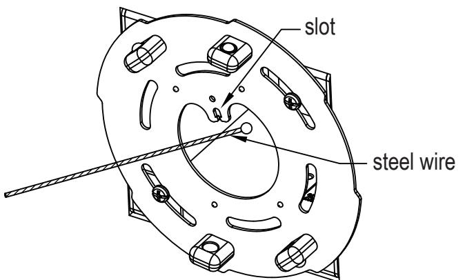
2. When ready to make the wire connections, first install the Safety Installation Cable from light fixture by pushing into the "key hole" in bracket..
