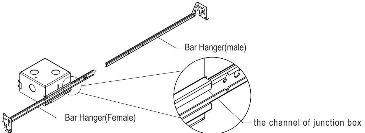
1. Before installation whole fixture ,Insert the Bar Hanger(Female) into the channel of junction box, then insert Bar Hanger(Male) the slot of Bar Hanger(Female) with right position.
