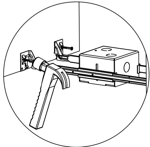
2. Put the Junction Box to the Wood Joist Properly.
