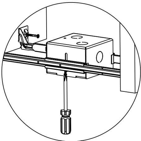
4. Moving the channels make the junction box to the properly place , then fix channel with screws.
